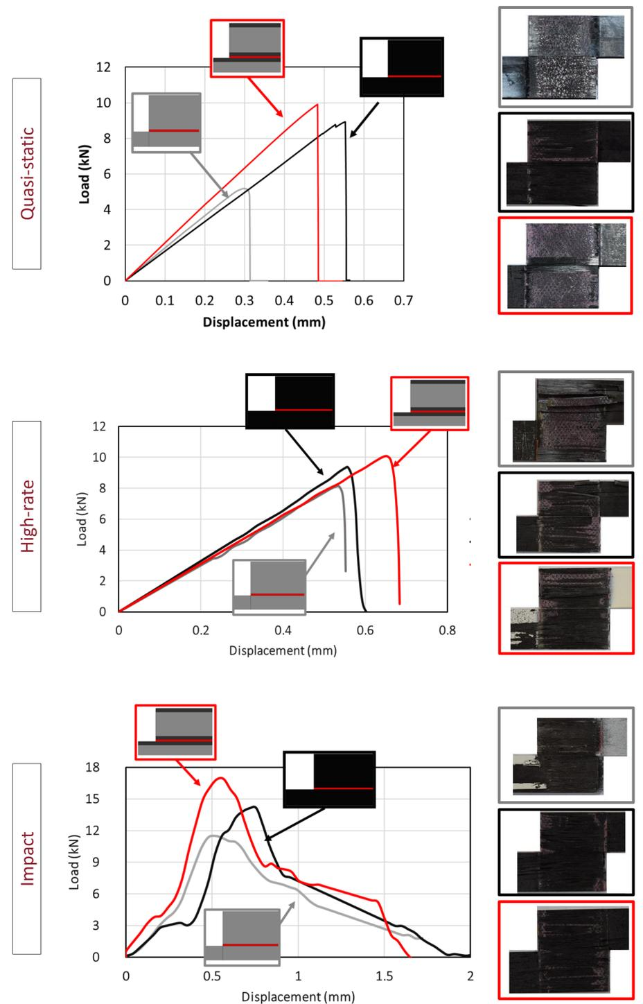
Figure 2 – Load-displacement of composite joint under different loading
