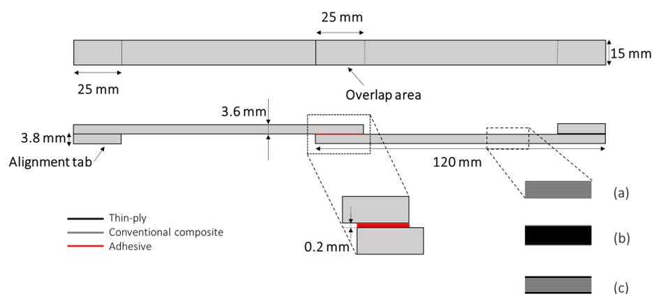
Figure 1 – Schematic design of (a) conventional composite, (b) thin-ply, and (c) hybrid joint (25% thin-ply) joint
